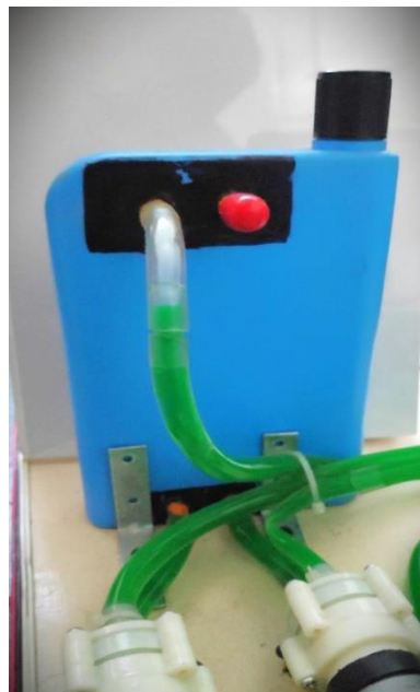
Figure 3.14: coolant reservoir used in model of project
